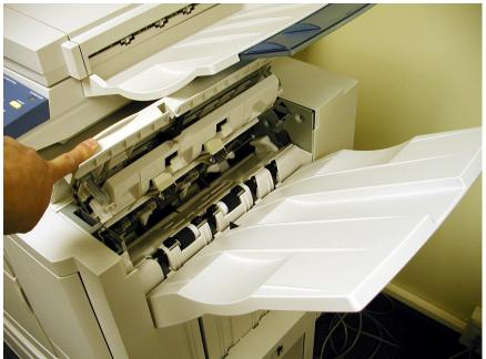
Figure 16 – The finisher's misfeed-access area.
